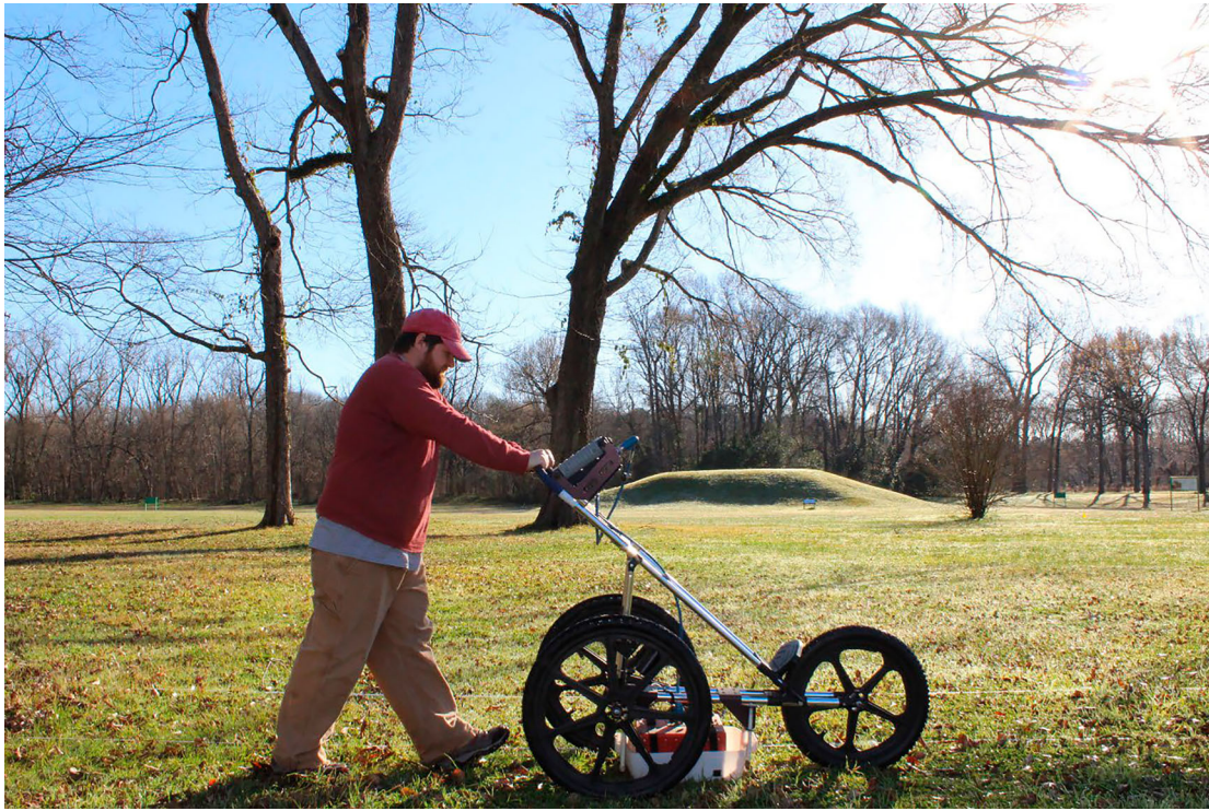
Figure 5. GPR survey at the Grand Village using the 400 MHz antenna with Mound B in the background, facing east.
